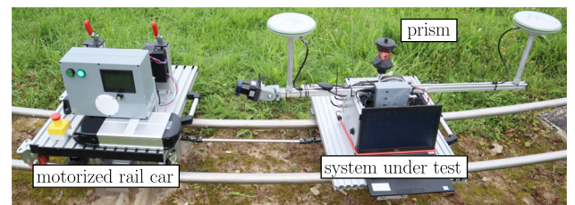
Figure 10: Motorized rail car with trailed rail wagon. The sensors under test can be mounted on the rail wagon. In addition, the rail wagon is equipped with a 360^\circ prism, which can be tracked with a total station to generate higher-order reference trajectories.
